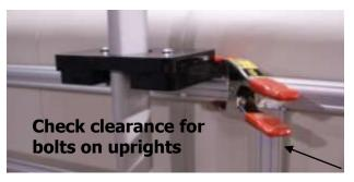
For most applications, place actuator bottom bracket onto edge cap of pontoon and drill (2) holes to secure using  $5/16'' \times 1''$  Hex Head bolt, 5/16'' Fender washer & nyloc nut.
