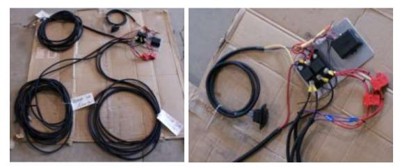
Run passenger side harness thru hole in floor located inside console, harness must be ran along the cross member on the underside of the floor. (The cross member will help protect the harness) Use zip ties and screws provided to fasten.
