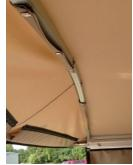
D. The curved crown bows have snap tracks on all four sides. Install the snap clips on the front, rear and middle crown bows where the flaps are sewn to the top canvas. Snap the flap snaps to the clips.
