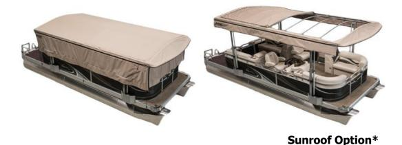
\*If you ordered a sunroof option on your Blue Water Top, there are footman loops and straps that are used to secure the sunroof back once it is open. These need to be installed by the customer.
