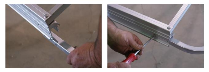
The rear hole has  $1\frac{3}{4}$ " truss head bolt, washer and spin nut.
