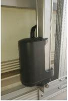
Optional mount method, if edge cap is not flat sided, use  $\#10 \times 1''$  screw to attach angle to edge cap then attach actuator over aluminum angle and drill (2) holes to secure using  $\frac{1}{4}''-20 \times 1''$  truss head bolt,  $\frac{1}{4}''$  Fender washer and lock nut.
