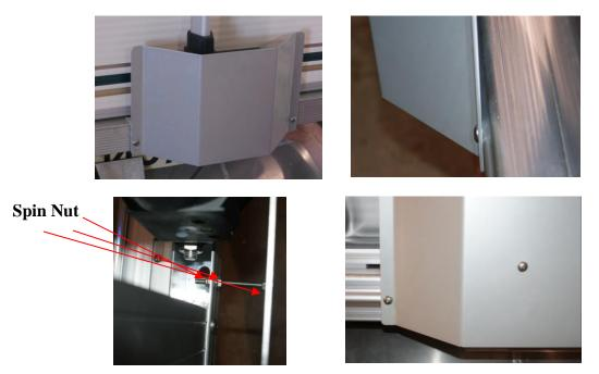
Optional: Drill a hole through the shield and the actuator bracket. Use  $\frac{1}{4}$ "-20 x 3" truss head bolt, (3)  $\frac{1}{4}$ " spin nuts. (Do 4 times, one for each actuator bracket)
