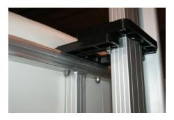
1. For most applications, place actuator bottom bracket onto edge cap of pontoon and drill (2) holes to secure using  $\frac{1}{4}$ "-20 x 1" truss head bolt,  $\frac{1}{4}$ " Fender washer and lock nut.
