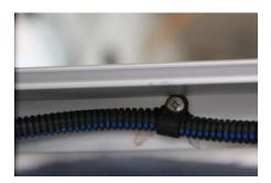
Run conduit with wiring through the  $\frac{1}{2}$ " hole in the actuator arm (which must be fully extended/up) and down through the channel and through  $\frac{1}{2}$ " hole in the bottom of the actuator. Then finally under floor and attach to existing bimini wire.
